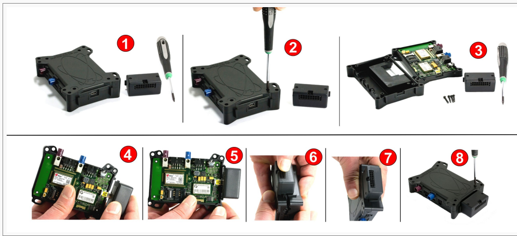
Figure 22: Mounting IOBOX-MINI to the FOX3 device.
