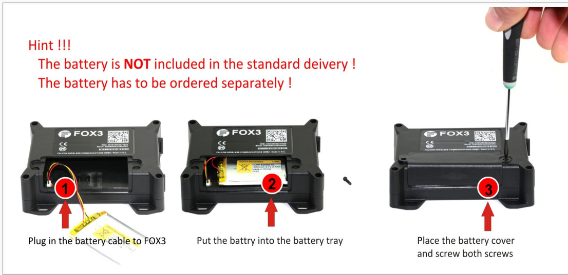
Figure 14.1: Connecting the battery to the FOX3
